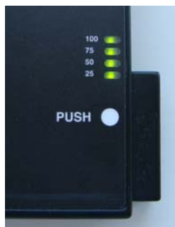
Figure 4-7. The built-in check button and diodes on the battery (UA1225).
